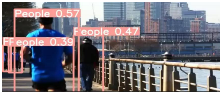
Figure 5 Pedestrian detection using CNN
