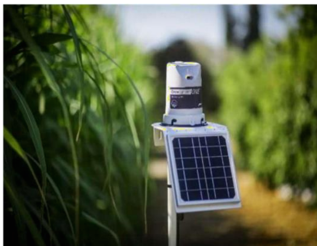
Figure 3: Weather Sensor (courtesy: Grow Sphere, Netafim)
