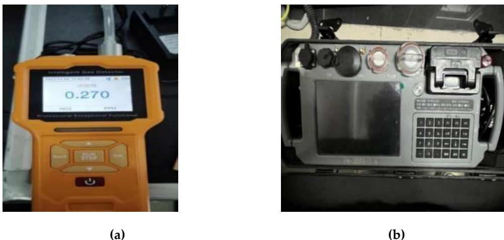
Figure 3.1 (a) Nitrogen Dioxide Flue Gas Analyzer; (b) Intelligent Smoke and Flue Gas Analyzer
